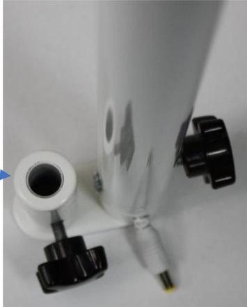
With the downtube directed it should be loosely fitted between the two metal clasps and then holes should be marked on the tube for where the safety bolt will go through; then remove the downtube and secure for drilling. A 7mm hole should be drilled through the downtube on both sides to allow the bolt to pass through.
